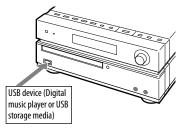
When USB cable connection is necessary, connect the USB cable supplied with the USB device to be connected.
